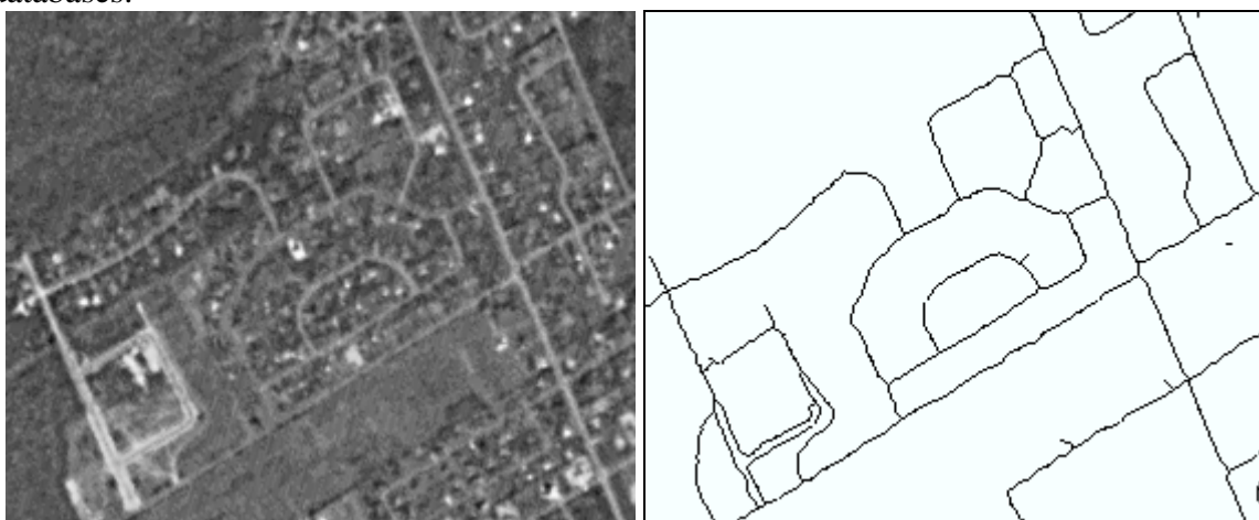
Figure 6 Road centerlines extracted from IRS pan image shown in Figure 2(a)
