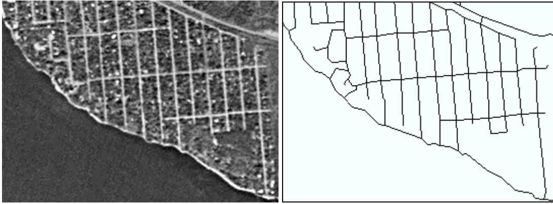
Figure 7 Road centerlines extracted from IRS pan image of urban area
