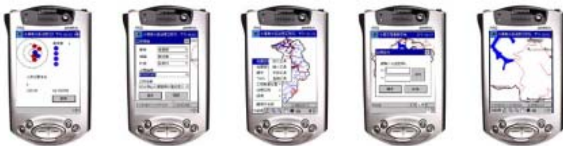
Figure 12 Mobilized Surveys Solution (Using GPS and PDA devices to take down disaster position and construction quality at on-site survey)
