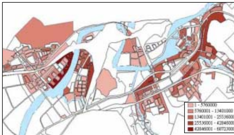
Figure 17: 3.1 meters flood damage map (block)
